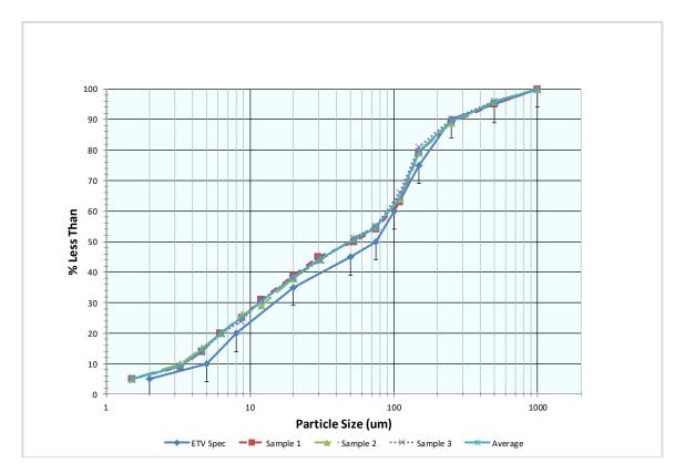
Figure 2 - The three sample average particle size distribution (PSD) of the test sediment used for the capture and scour test compared to the specified PSD
