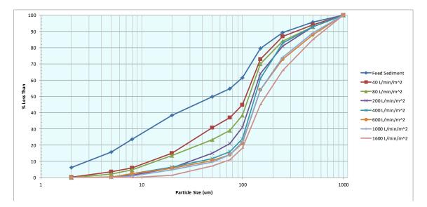
Figure 3 - Particle size distribution of sediment retained in the Downstream Defender<sup>®</sup> OGS in relation to the injected test sediment average
