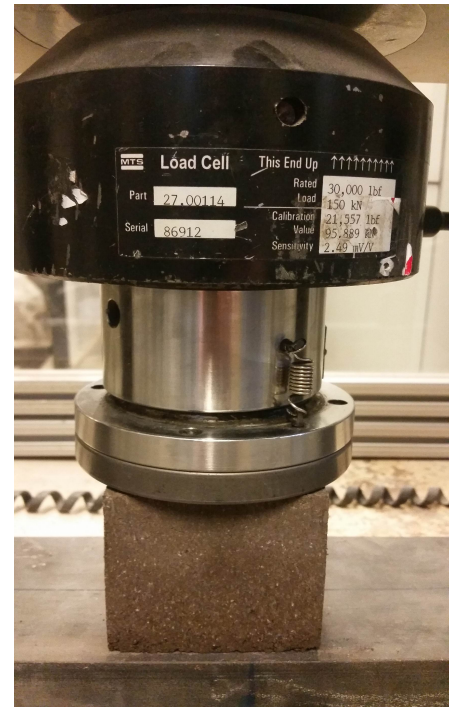
Observation of a compressive strength test of novel concrete replacement
